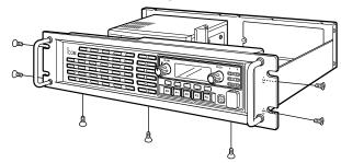
3 Disconnect the control cable from the channel module (original), then remove the front panel.
