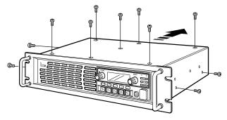
② Remove 3 screws from bottom and 2 screws each from both sides of the repeater.
