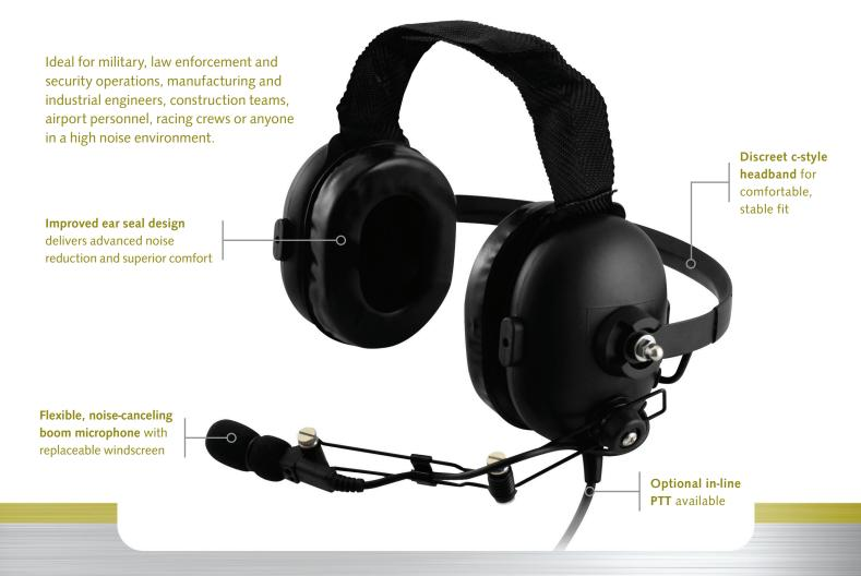
OTTO **Behind-the-Head heavy duty headsets** are Mil-Spec and IS/ATEX certified and deliver comfort, reliability and protection. Fitting snugly to the head, the headset can be worn comfortably under a helmet. It offers a certified noise reduction rating (NRR) of 24dB and provides high clarity audio and additional hearing protection necessary for consistent, clear communication in extreme noise environments.
